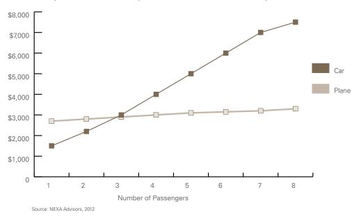
States have developed cost comparisons to other modes of transportation to justify use of the state aircraft, such as the cost comparison shown above developed by the state of Idaho
